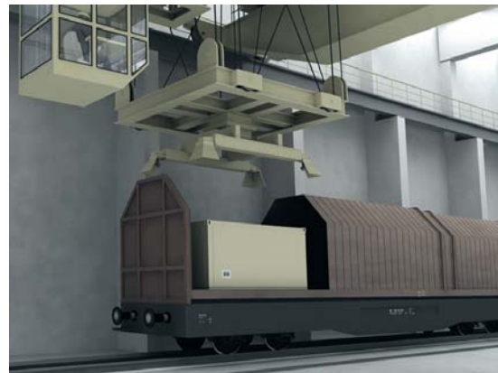
Fig. 3: Waste packages arriving in the repository's surface facilities will be reloaded from the train or truck to local transport vehicles [7].
